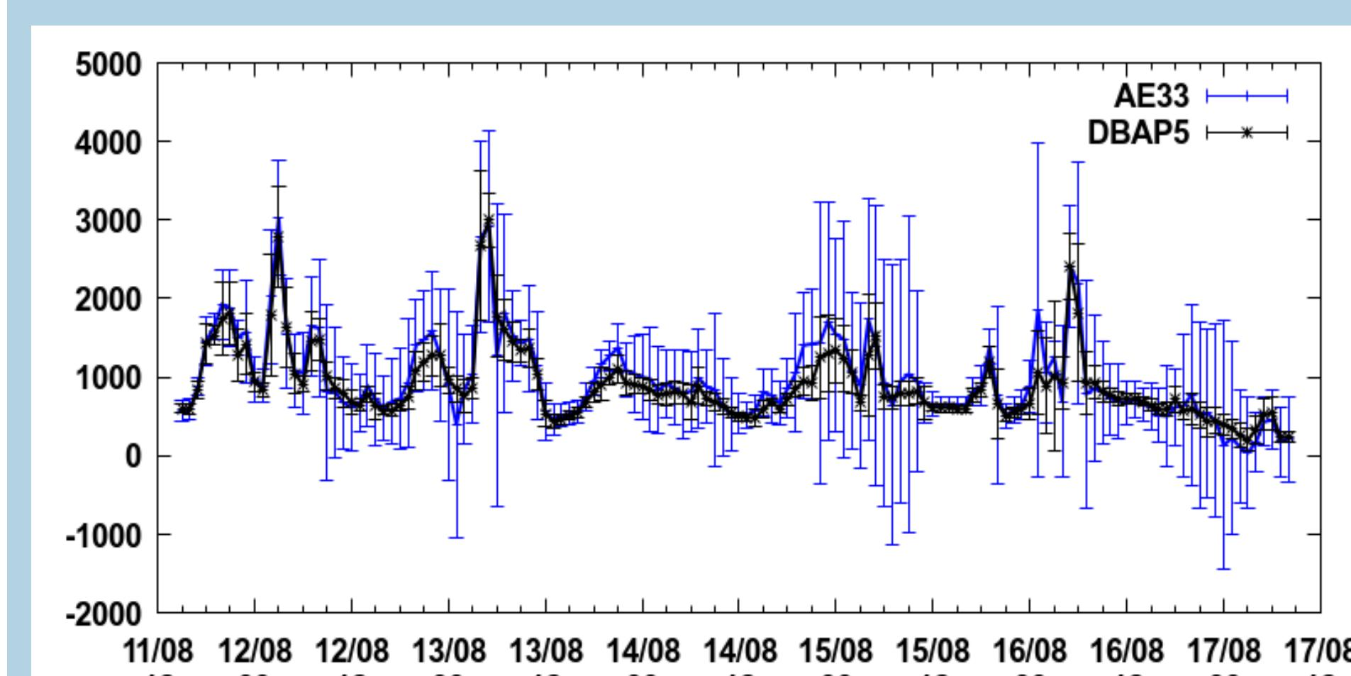
One hour averaged data has been used to compare DBAP5 and AE33 measures. Correlation is very good, Comparing the SD, the
