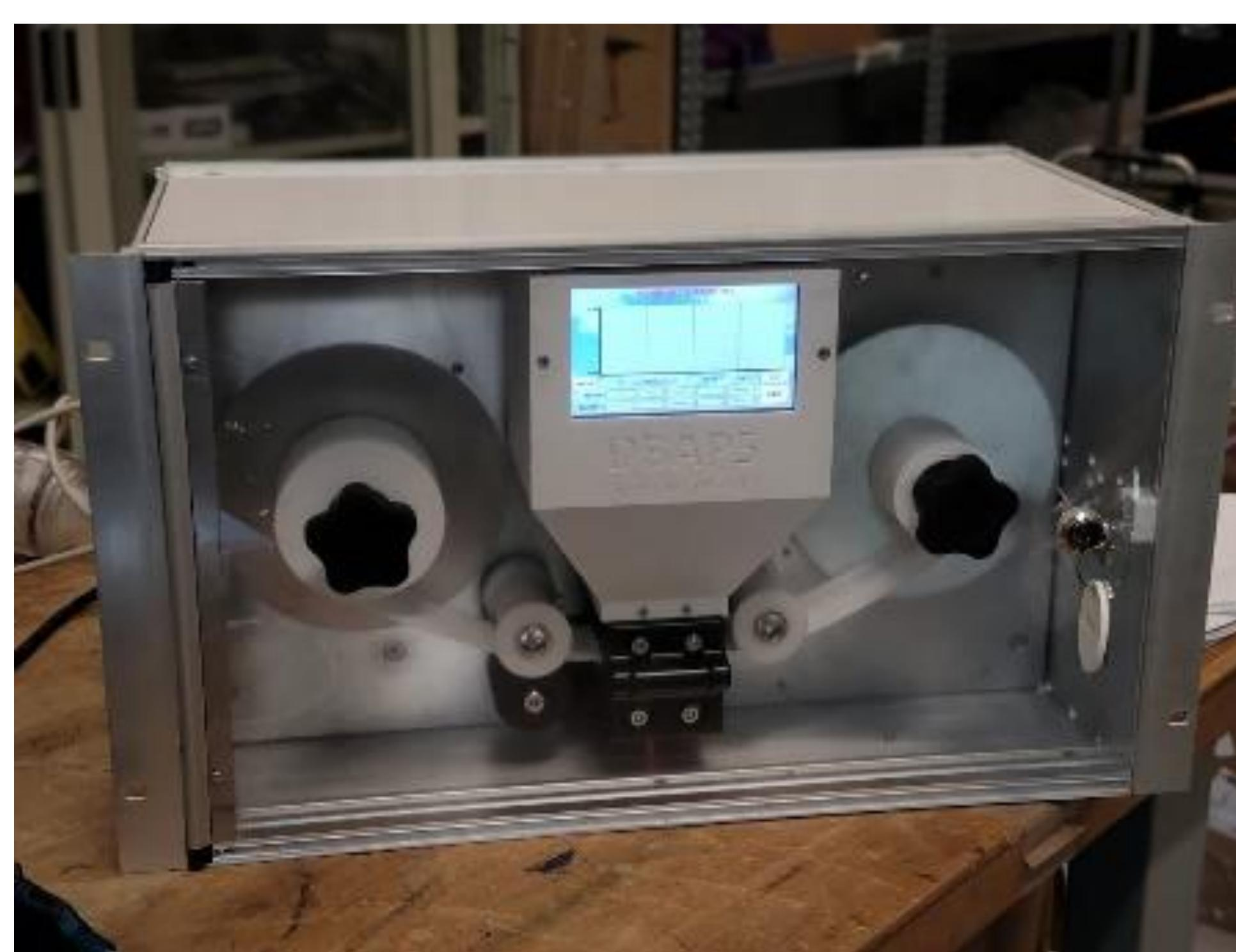
Measuring the variation in filter light transmission at increasing particle load it evaluate the attenuation coefficients, then converted in the absorption coefficient by applying the appropriate filter correction equations.
