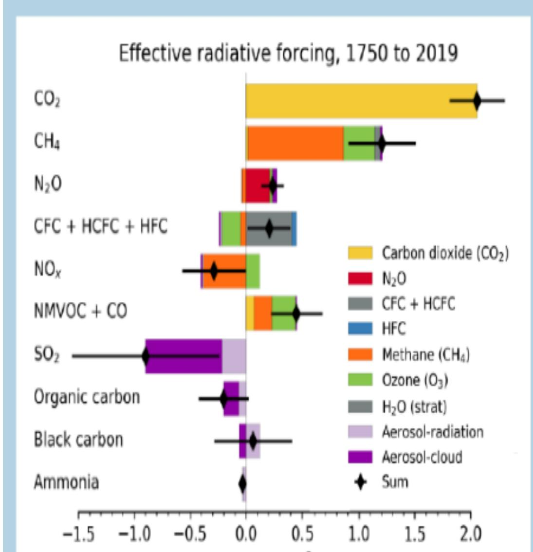
By strongly absorbing solar radiation and reducing albedo, when deposited on snow and ice, BC has a warming effect on climate [1], the quantification of which is still uncertain.
