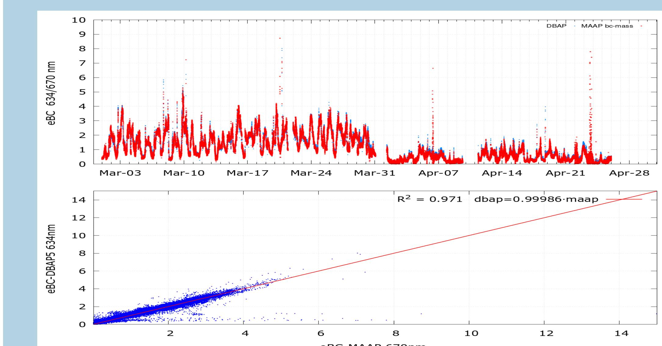
One-minute data have been compared for two months. The results show a powerful agreement between two instrumental setup.
